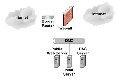
Figure 7.3: Three Interface Firewall DMZ
