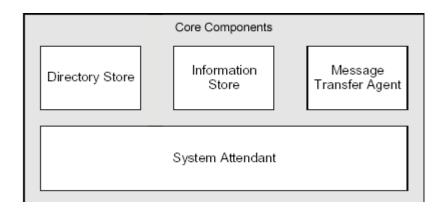
Figure E.1: Exchange Server Core Components
