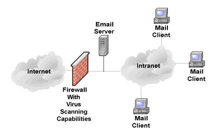
Figure 6.1: Virus Scanning Implemented on Firewall
