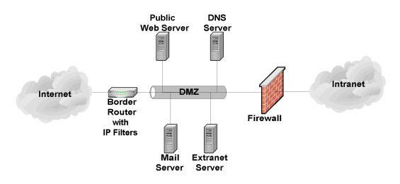
Figure 7.1: Simple Single Firewall DMZ
