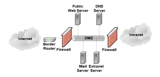
Figure 7.2: Two Firewall DMZ
